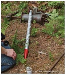
Sand point (driven) wells are constructed using a cylindrical pipe with a screened/perforated section and pointed end that is hammered into the ground. They are usually shallower than drilled wells, with a smaller diameter steel casing (e.g. 2 inches)
