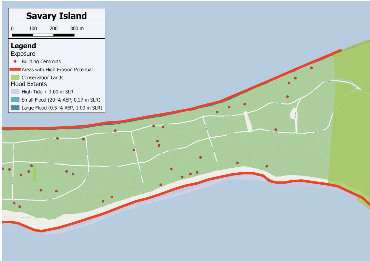
Figure 4-8: Map showing the illustrative archetype area for “Island Sanctuary”. The red line denotes a “very high” erosion potential. Note that address points are indicative only and do not necessarily represent the presence of a home.
